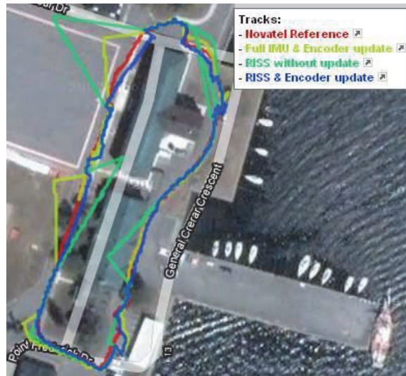
Fig. 6. Three solutions and reference for first trajectory: Red for reference, Yellow for KF using full IMU with velocity updates, Green for KF using RISS without updates, Blue for KF using RISS with velocity updates.
